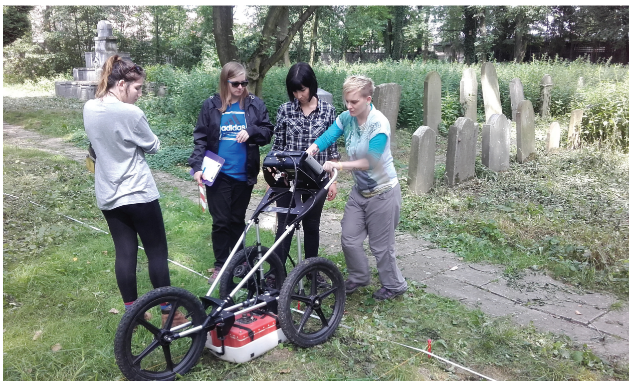
Figure 1. Ground Penetrating Radar survey at Oświęcim cemetery in Poland aimed at locating unmarked individual burials and mass graves (Copyright Centre of Archaeology).
