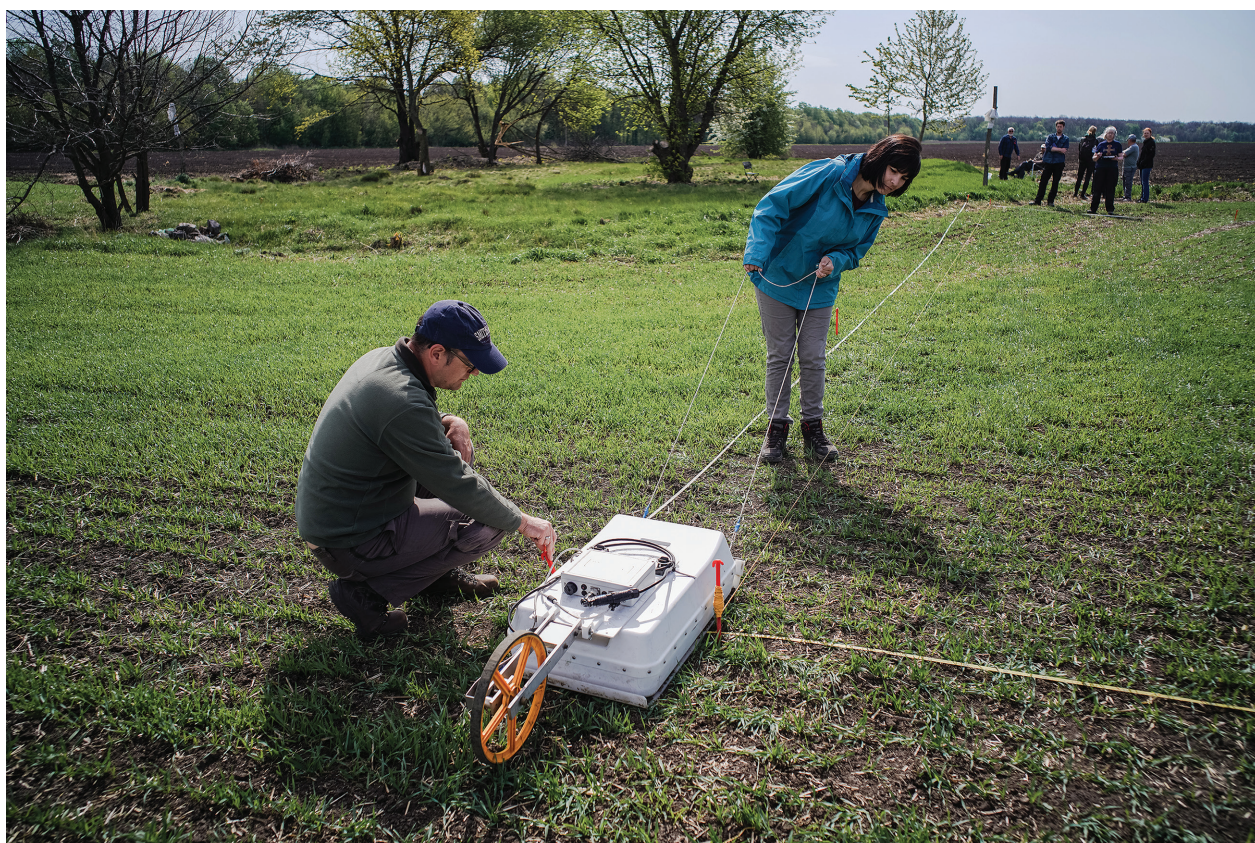
Figure 3. Ground Penetrating Radar survey in rural Ukraine aimed at locating unmarked mass graves under rabbinical supervision (Copyright Centre of Archaeology).
